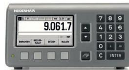
The ND 280 evaluation unit for one axis is suitable for measuring and inspection stations, as well as simple positioning tasks. The universal encoder input permits the connection of all incremental encoders with  $11 \mu\text{App}$  and  $1 V_{\text{pp}}$  signals, and absolute encoders with the EnDat 2.2 interface from HEIDENHAIN.
