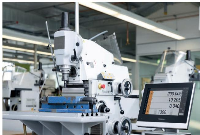
Distance-to-go mode comes to your aid during positioning tasks. With it, you can easily and reliably arrive at the next position by simply moving the axes until the display reads zero. This feature is particularly useful during the execution of programs.
